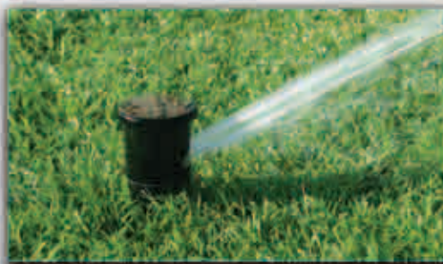
Gear Driven Rotor type heads must run three times as long, to get the same coverage as a "fan" type pop up head.
